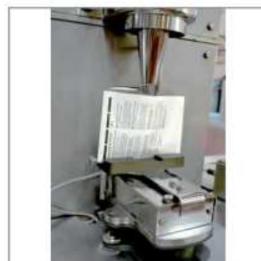
Fine filling of sachets (pharmaceutical application)
